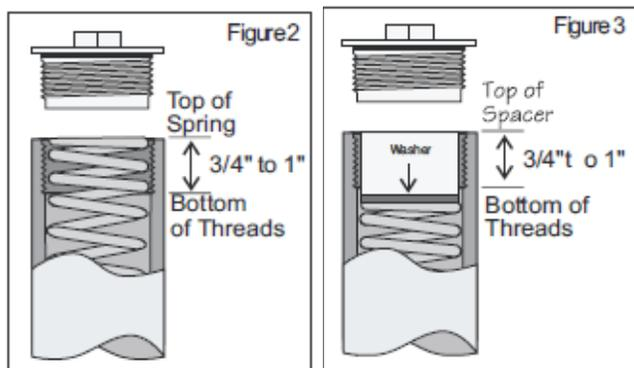
Also check the Notes in the enclosed Application Supplement, the stock spacer in some cases can be modified to fit. If making a spacer, we recommend PVC pipe that is the approximate diameter of the fork springs but will still fit inside the fork tubes. **Warning:**
