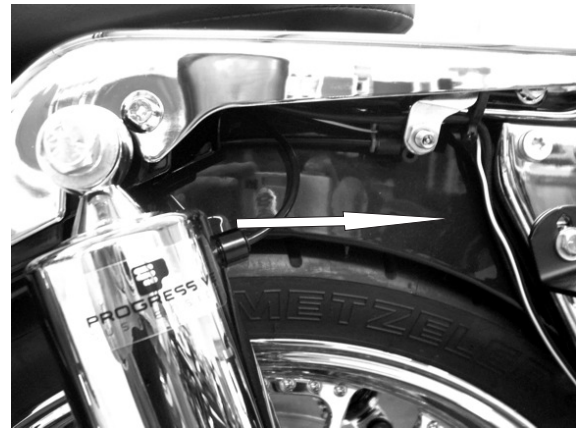
Photo 2 Install shocks so air fittings points rearward.
