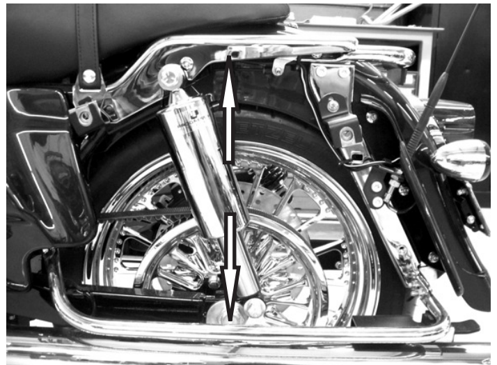
Photo 5 The difference in measurements between the axle and the fender rail with the suspension fully extended and then with rider(s) on the bike is your Ride Sag. This difference should be 1.0” - 1.2” for maximum ride comfort.
