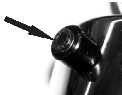
Photo 4 Push in the collar to remove the plug or air lines.
