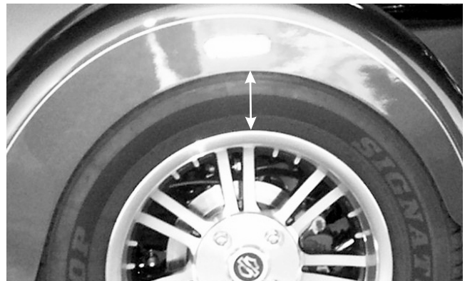
Photo 5 The difference in measurements between the top of the rim and the fender with the suspension fully extended and then with rider(s) on the bike is your Ride Sag. This difference should be .80" - 1.2" for maximum ride comfort.
