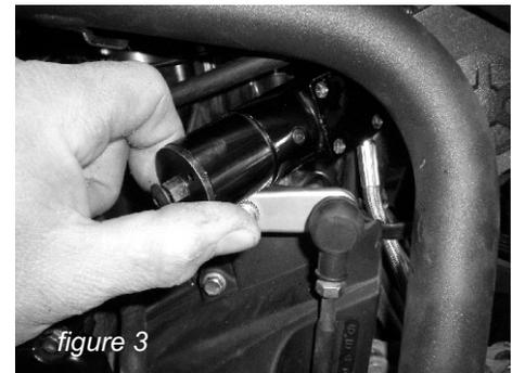
To adjust the ride height, simply turn the adjuster knob clockwise (looking at it from the front of the bike) to increase the height and counterclockwise to reduce it. See main instructions for procedure of achieving optimum ride height.
