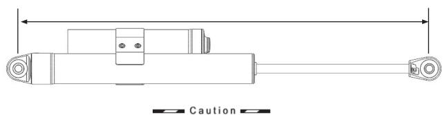
• Adequate full front suspension travel must be checked to ensure the vehicle bottoms out on the front bump stops before the shock reaches its metal to metal compressed length. Lower the frame of the vehicle (or raise the axle) until it bottoms and fully compresses the front bump stops. Referring to **figure 2** below, ensure that the distance between the upper and lower shock mounting points is greater than the stated values for your specific configuration.
